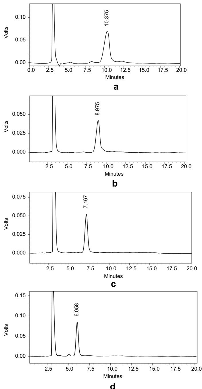
**Fig. 2.** HPLC profile of purified oligosaccharides liberated from wheat bran SP: (a) WO-1; (b) WO-2; (c) WO-3; (d) WO-4. Eluent system used is acetonitrile:water (75:25) at a flow rate of 0.7 ml/min. WO-1, WO-2, WO-3 & WO-4 represent the four major oligosaccharides liberated from wheat bran soluble polysaccharides.
