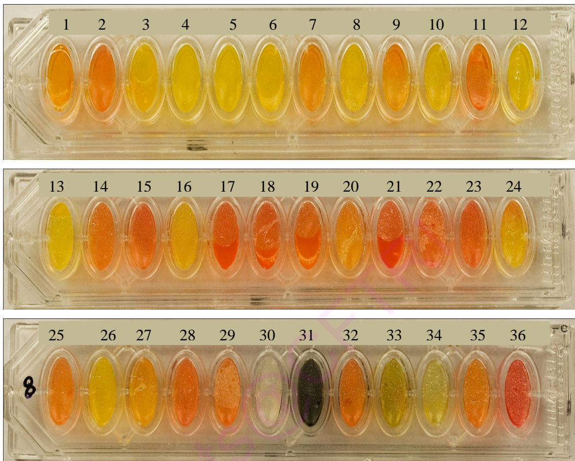
Fig 5.5 (a) Carbohydrate fermentation test of the probiotic LAB isolate Cu8 (wells numbered from 1-35 correspond to carbohydrates mentioned in Table 5.5 in the same order and well number 36 represents control)
