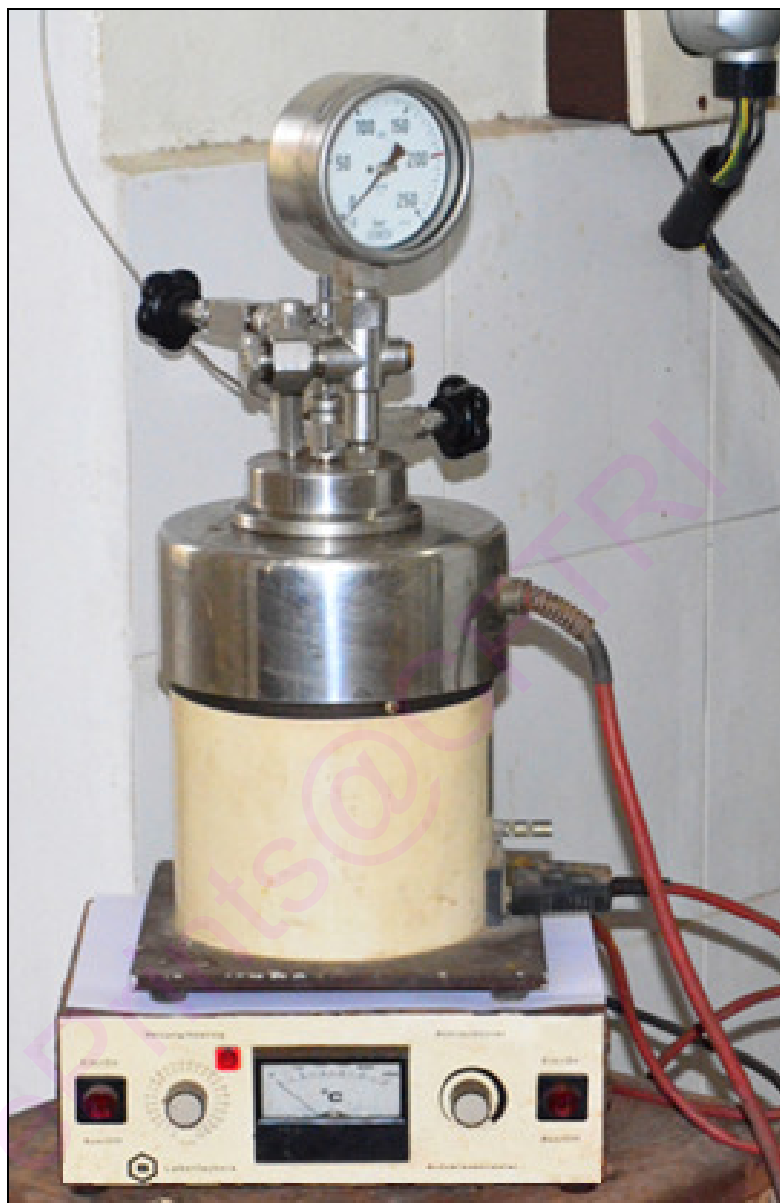
Fig. 6.2. Reaction setup for glycosylation of thymol in supercritical CO 2
