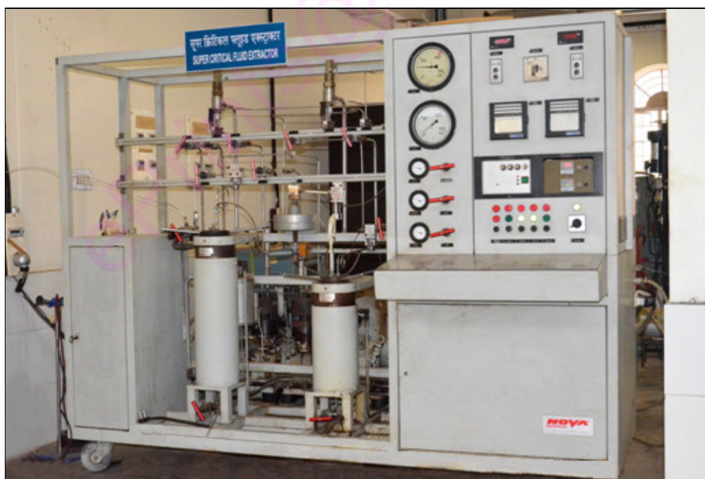
Fig. 2.6. Supercritical carbon dioxide extraction plant.
