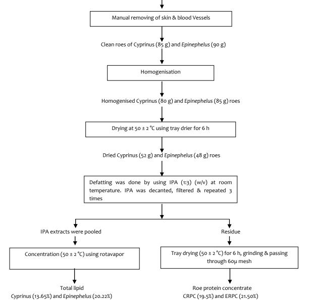
Fig. 1. Flowchart depicting the unit operations involved in the preparation of roe protein concentrates and total lipid
