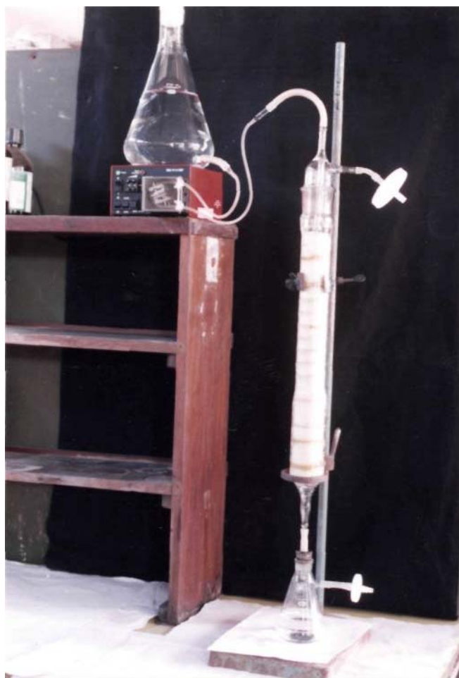
Figure 3.41. Packed-bed reactor (1 L) used for studies on continuous production of capsaicin from Capsicum frutescens cells immobilized in polyurethane foam.
