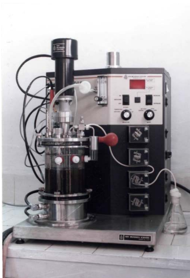
Figure 3.31. Stirred tank bioreactor (2 L) used for studies on growth and anthocyanin production from Daucus carota cell culture.
