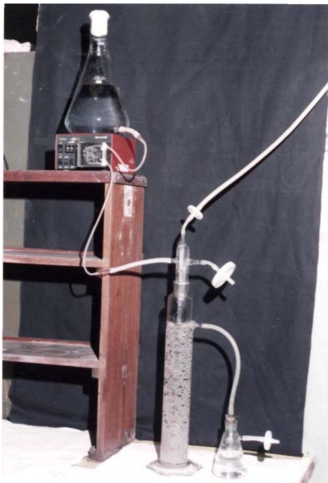
Figure 3.38. Bubble column reactor (1 L) used for studies on continuous production of capsaicin from Capsicum frutescens cells immobilized in alginate beads.
