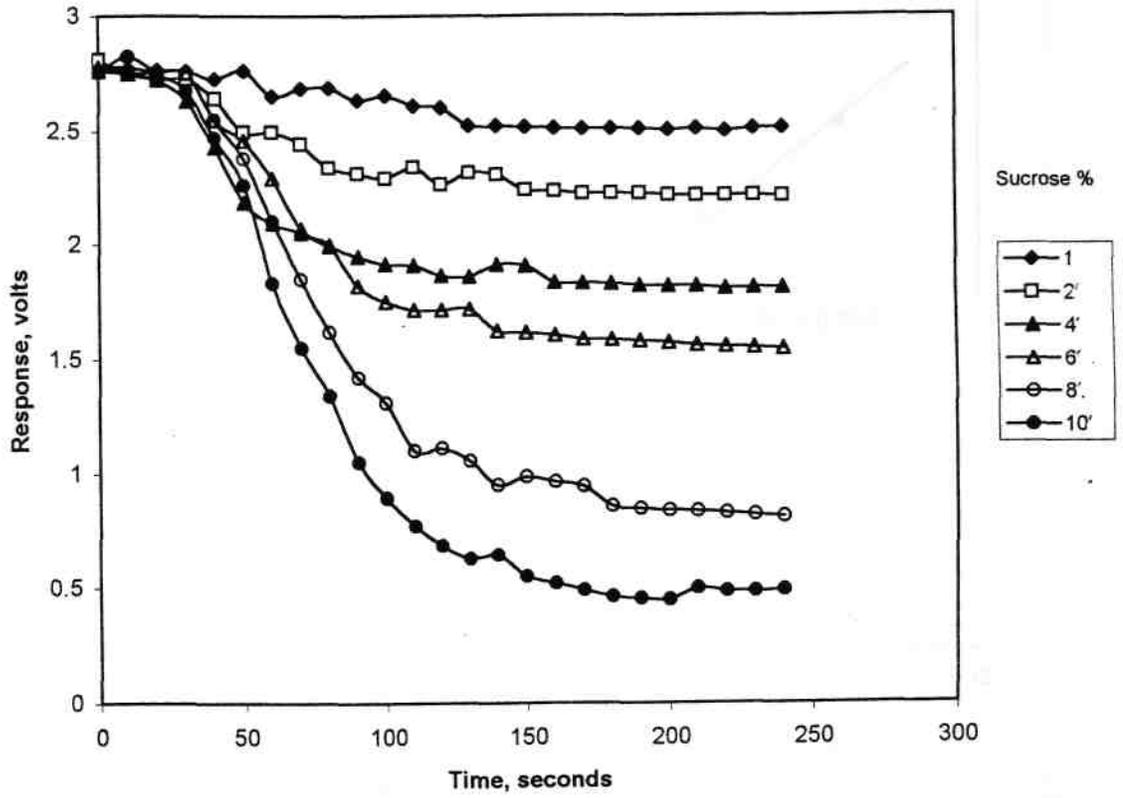
Figure 2.12.3 Response curve for various concentrations of sucrose with sucrose biosensor
