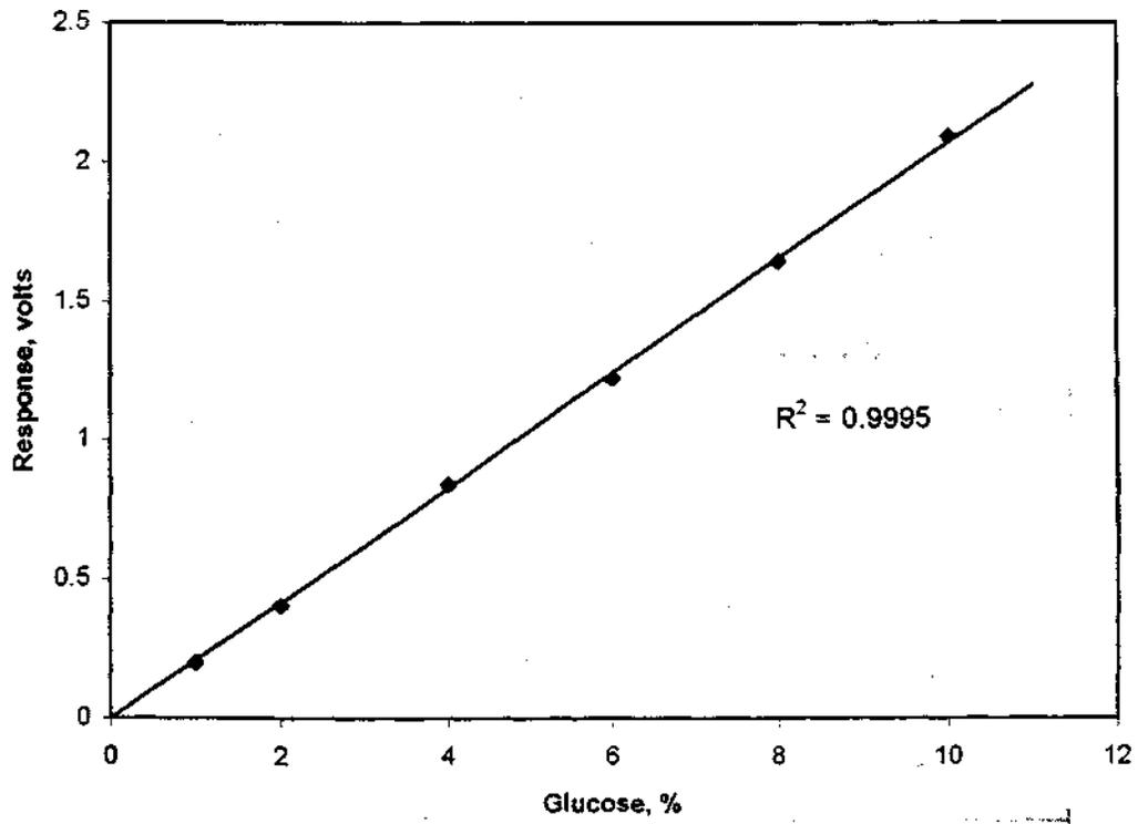
Figure 2.12.2 Calibration graph for the various concentrations of glucose with glucose biosensor
