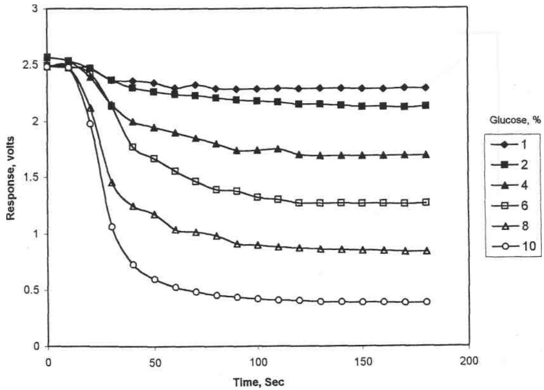
Figure 2.12.1 Response curve for various concentrations of glucose with glucose biosensor
