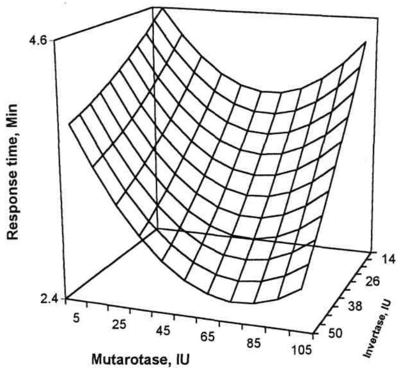
Figure 3.7.1 Response surface plot showing the effect of mutarotase and invertase on the response time. GOD is constant at 1 IU level.
