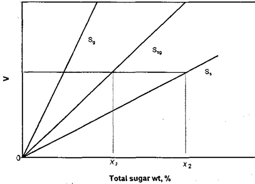
Figure 4.4.5 Schematic plot of voltage response of the sucrose electrode against various concentrations of glucose ( $S_g$ ), mixture of glucose and sucrose ( $S_{Sg}$ ) and sucrose ( $S_s$ ).
