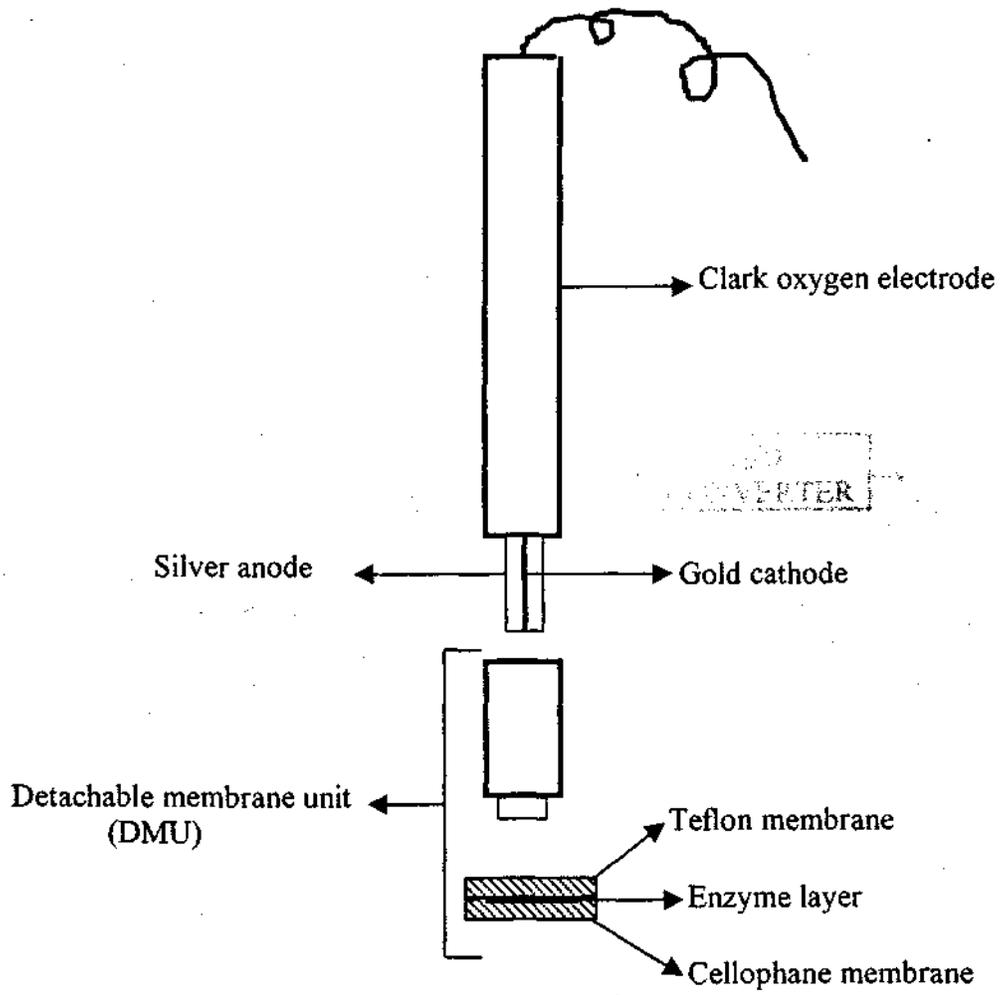
**Figure 2.8.1 Schematic diagram of the enzyme electrode used for the stability studies**
