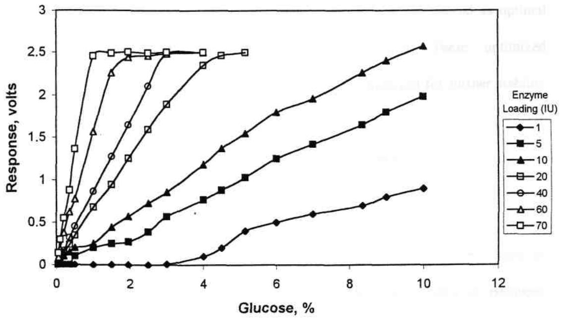
Figure 3.5.1 Effect of enzyme loading (IU) on the biosensor response for glucose
