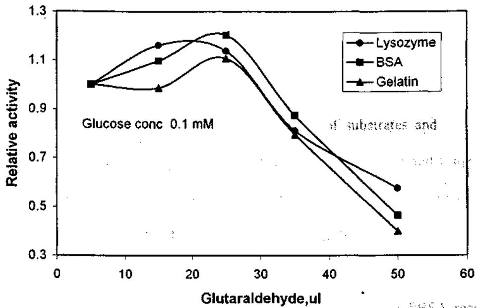
Figure 3.3.1 Effect of glutaraldehyde concentration on the biosensor response for the GOD immobilized with various PBSAs.
