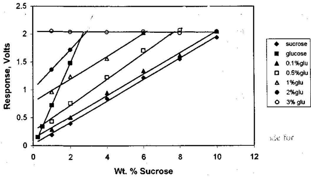
Figure 4.4.2 Steady state voltage response against sucrose concentration in mixtures containing varying concentrations of glucose.
