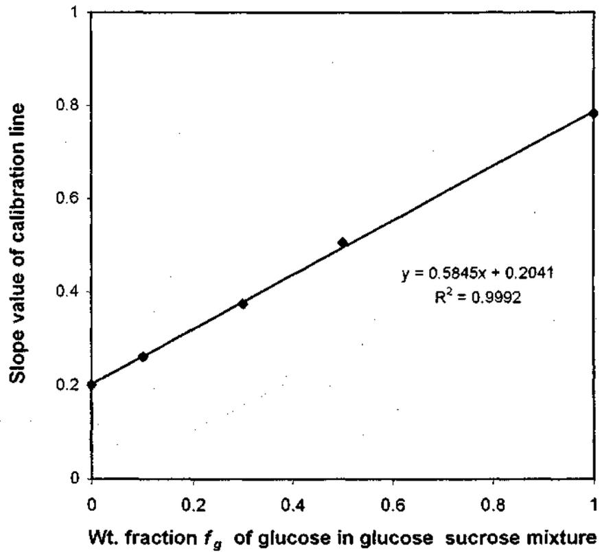
Figure 4.4.4 A plot of slope values from fig. 4.4.3 versus the weight fraction ( $f_g$ ) of glucose.
