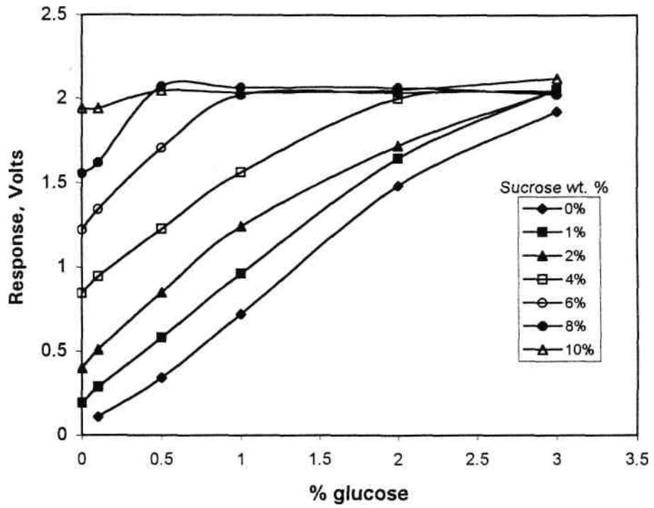
Figure 4.4.1 Steady state voltage response versus glucose concentration in a mixture containing different percentages of sucrose.
