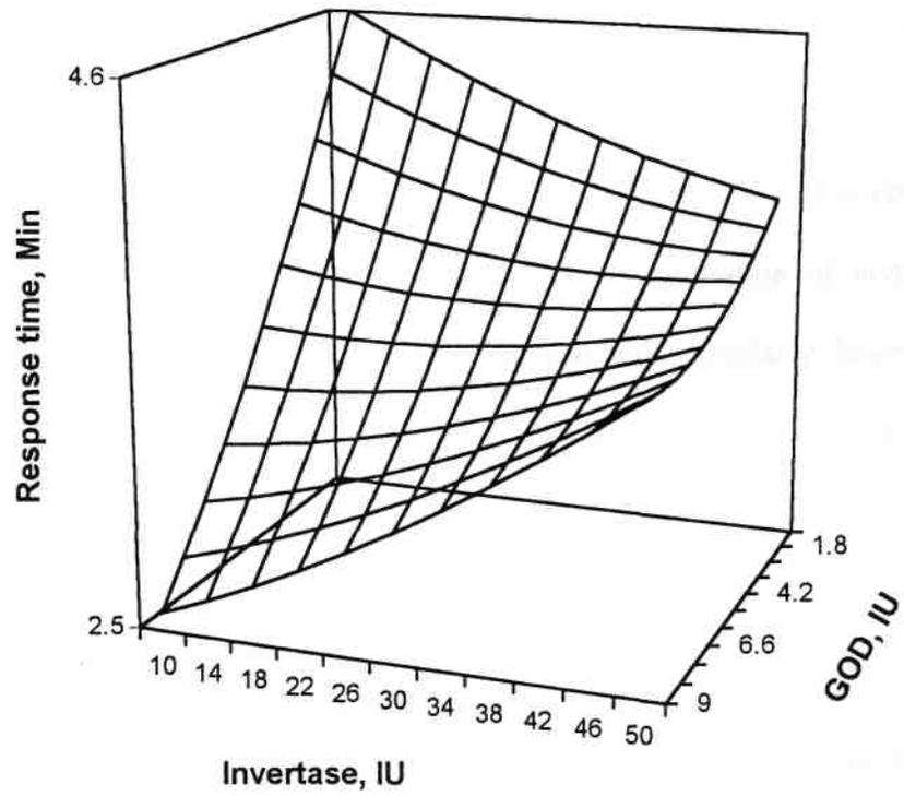
Figure 3.7.3 Response surface plot showing the effect of invertase and GOD the response time. Mutarotase is constant at 5 IU. level.
