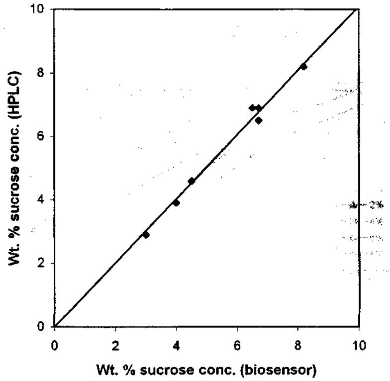
Figure 4.3.2 Sucrose concentration values predicted by equation (4.1) using the biosensor for various food samples plotted against those obtained by HPLC method.
