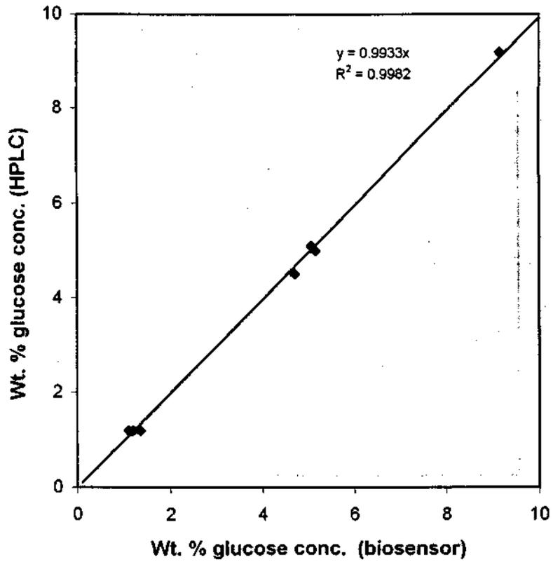
Figure 4.3.1 Glucose concentration values predicted by using the glucose biosensor for various food samples plotted against those obtained by HPLC method.
