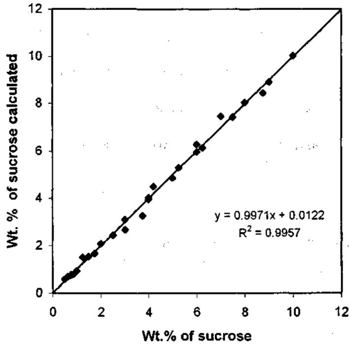
Figure 4.2.1 Sucrose concentration calculated by equation (4.1) against the actual concentration initially taken in the glucose and sucrose mixture.
