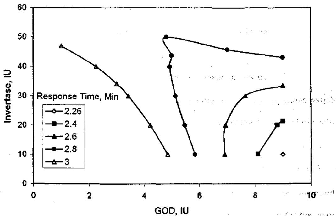
Figure 3.7.4 Contour plot showing the ranges of invertase and GOD to obtain various constant response time values. Mutarotase value is constant at 40 IU.
