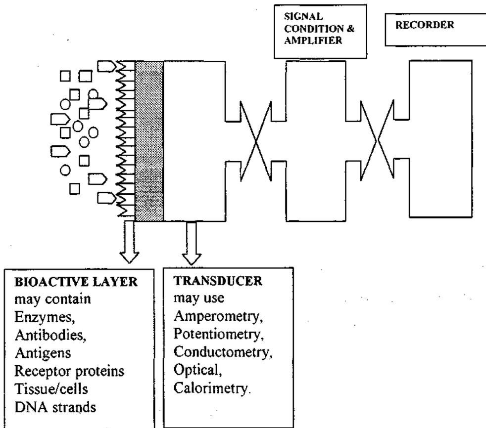
**Figure 1.2 A generalized scheme of biosensor configuration.**
