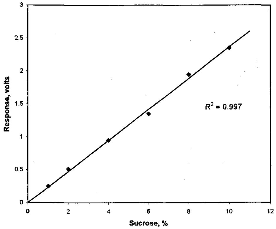
Figure 2.12.4 Calibration graph for the various concentrations of sucrose with sucrose biosensor
