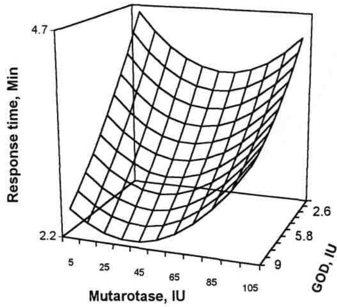
Figure 3.7.2 Response surface plot showing the effect of mutarotase and GOD on the response time. Invertase is constant at 30 IU level.
