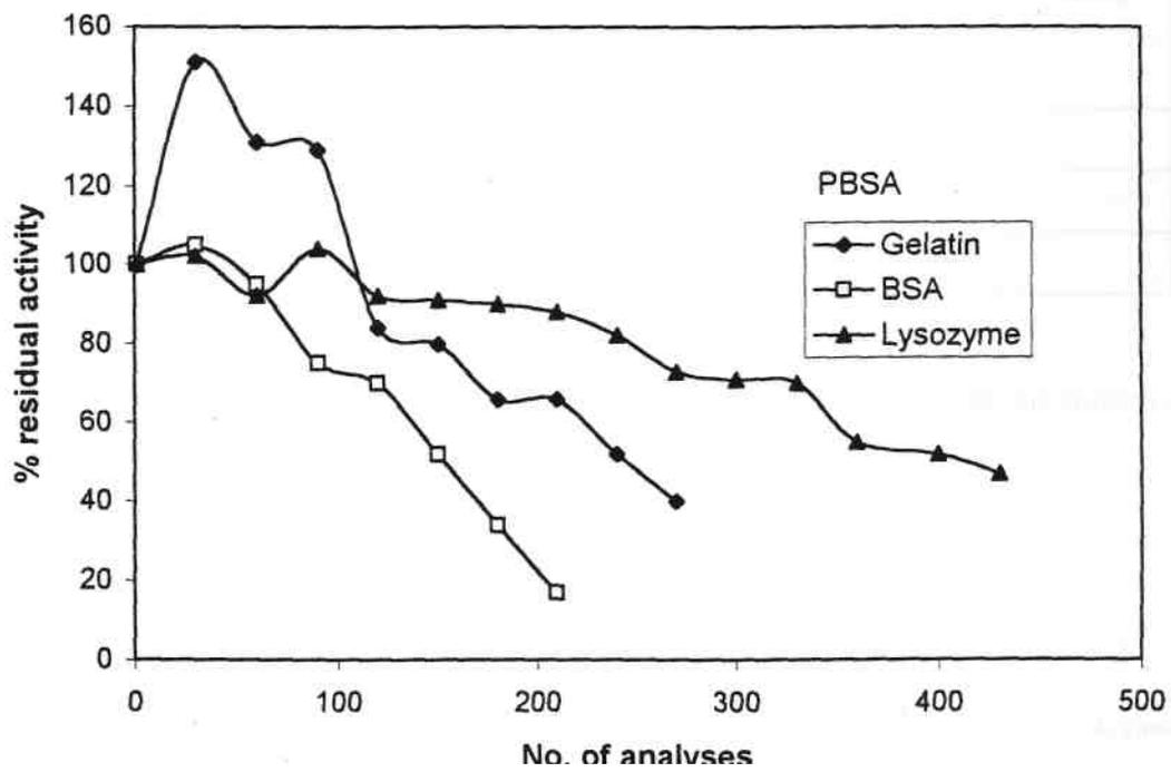
Figure 5.2.1.1 Residual activity after repeated sucrose (10 %) analysis with biosensor using GOD immobilized with different PBSA at pH 6.0.
