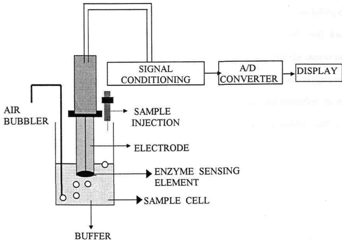
Figure 2.8.2 Schematic diagram of the biosensor device for the estimation of glucose and sucrose
