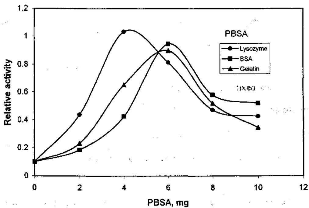
Figure 3.4.1 Effect of PBSA concentration on the biosensor response for glucose(0.1mM)
