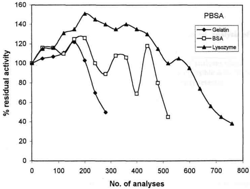
Figure 5.1.1 Residual activity after repeated glucose (3%) analysis with biosensor using GOD immobilized with different PBSA.
