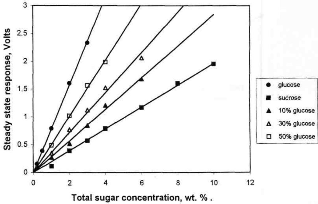
Figure 4.4.3 Steady state voltage response of the sucrose electrode against total sugar concentration for different weight fractions of glucose in the glucose and sucrose mixture.
