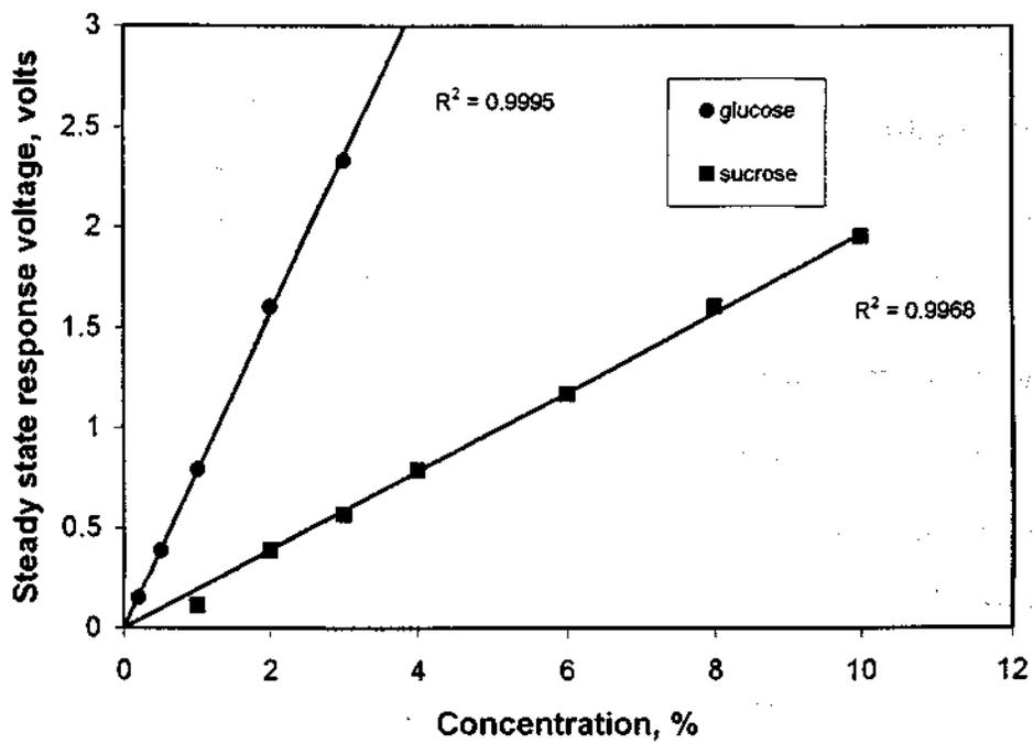
Figure 4.1.2.1 Voltage response of the sucrose electrode for pure glucose and sucrose.
