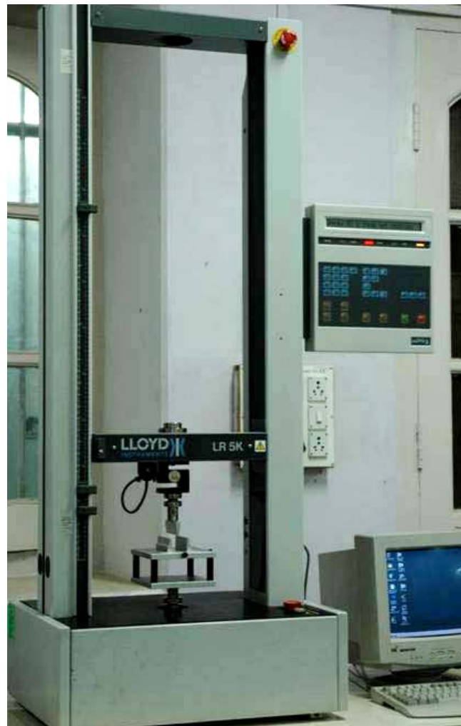
Fig. 18. LLOYDS texture measuring system
