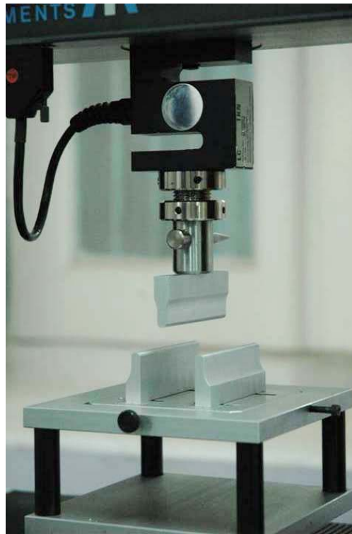
Fig. 19. Aluminum probe attached to LLOYDS Texture analyzer for measurement of spaghetti strength
