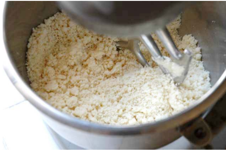
Fig. 14. Hobart mixer used for premixing of semolina and water to make a uniform dough
