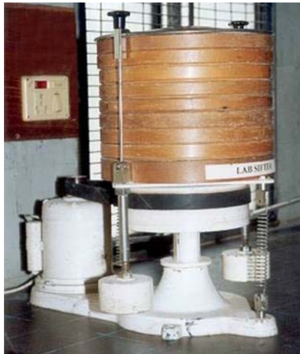
Fig. 10. Buhler laboratory sifter used for determination of semolina particle size
