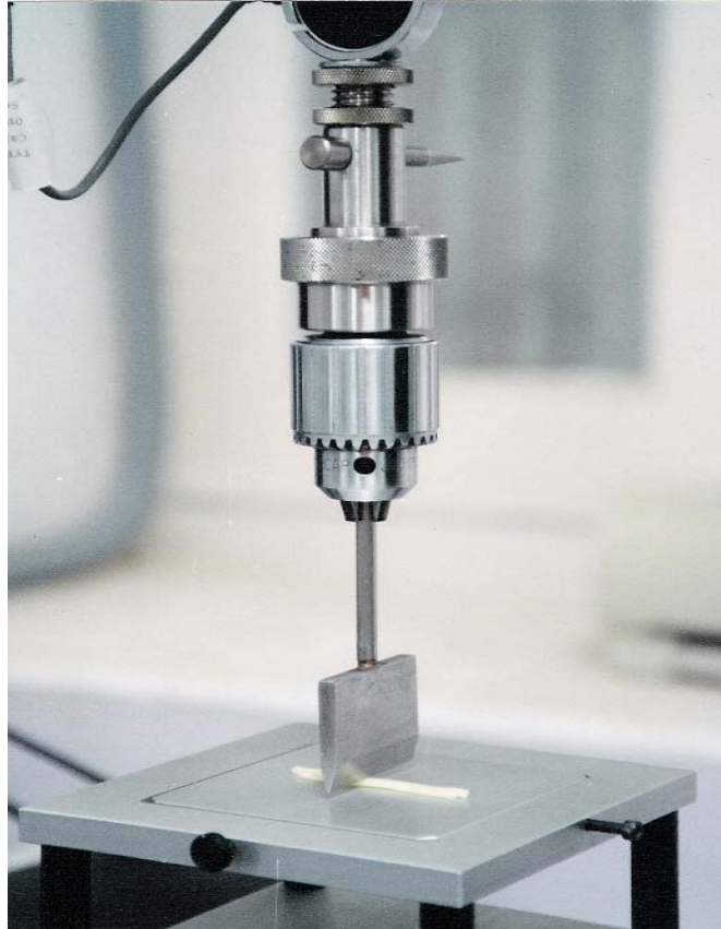
Fig. 20. Aluminum shearing blade attached to LLOYDS texture analyzer for measurement of spaghetti firmness
