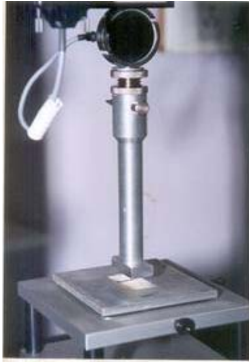
Fig. 21. LLOYDS texture analyzer with special plunger and sample holder for instrumental assessment of cooked spaghetti stickiness
