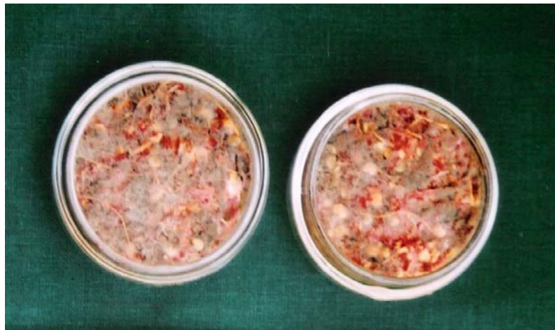
Fig.12. Chilli (powder) after exposure (RH 92 %).
