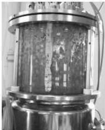
Fig. 24. A. Chemap<sup>R</sup> Fermentor used for scale-up studies
