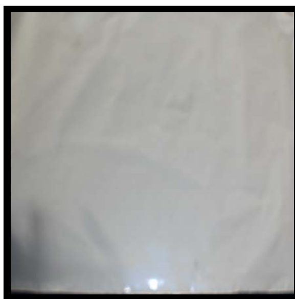
Fig. 23: Film (solvent caste) prepared from PHA obtained from Bacillus sp 256
