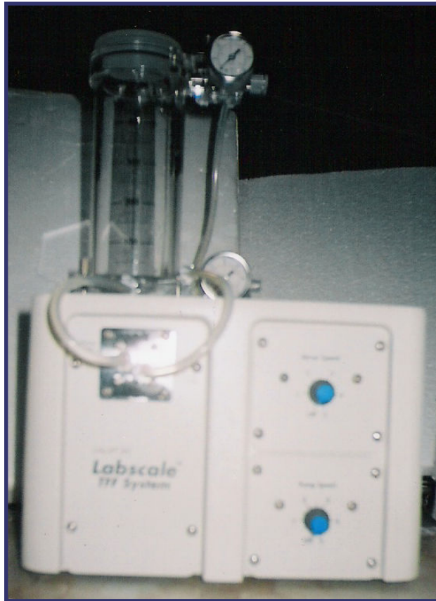
Fig. 4B.1 Tangential Flow Filtration (TFF) system used for ultrafiltration
