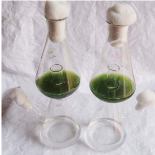
Fig 13. Experimental set up showing the CO 2 supplementation for Dunaliella bardawil cultures adopting two-tier flask method.
