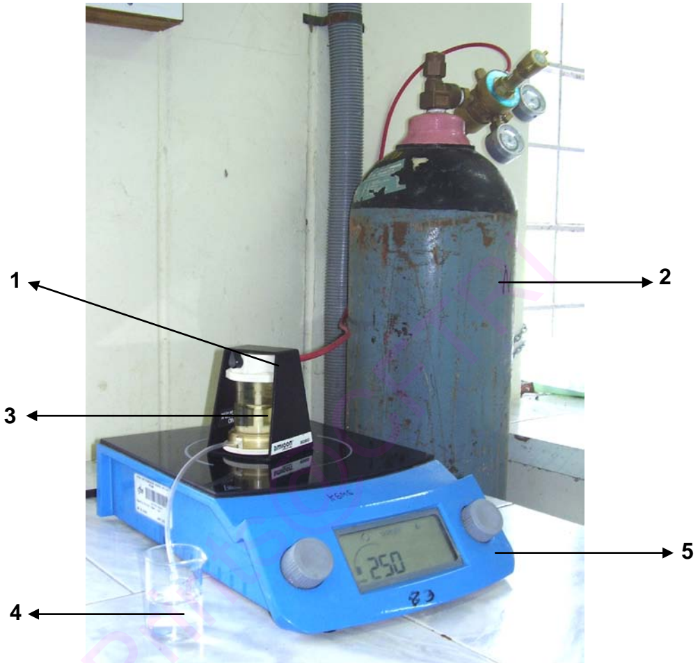
Figure 5A.1: Photograph of ultrafiltration stirred membrane cell. (1. membrane cell; 2. nitrogen cylinder; 3. retentate; 4. permeate; 5. magnetic stirrer)
