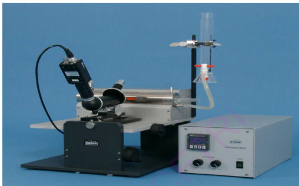
Figure 2A.1. Photograph of Spinning drop tensiometer
