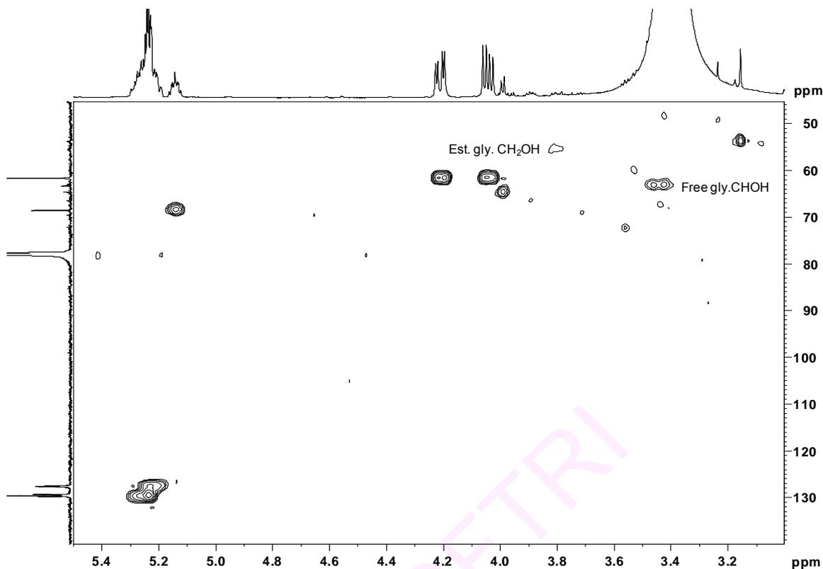
**Fig. 5.4** Esterified glycerol portion of the spectrum for 3.1-5.5 ppm of the permeate
