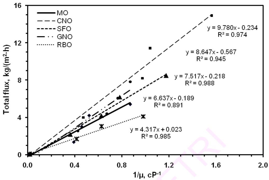
**Fig. 4.6** Influence of feed viscosity on total flux of undiluted and hexane-diluted oils
