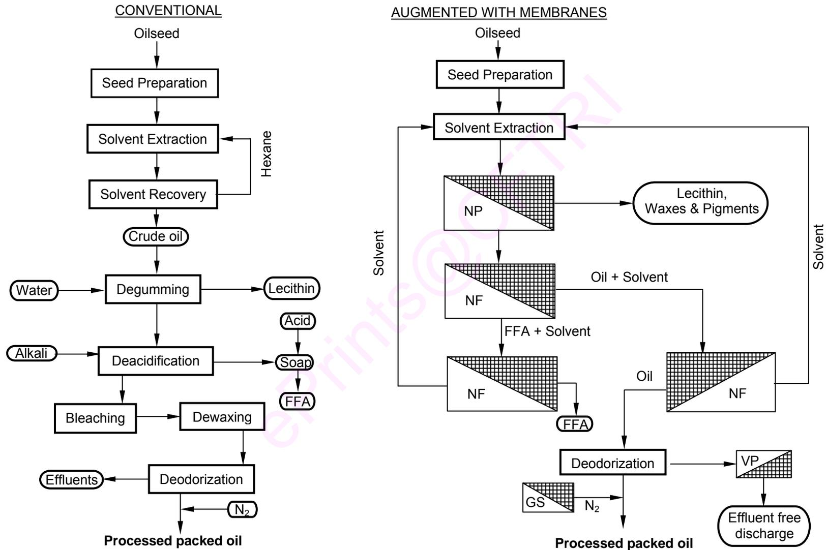
**Fig. 1.1** Typical conventional processing of vegetable oils and processing augmented with membranes (Modified based on Cheryan, 1998)
