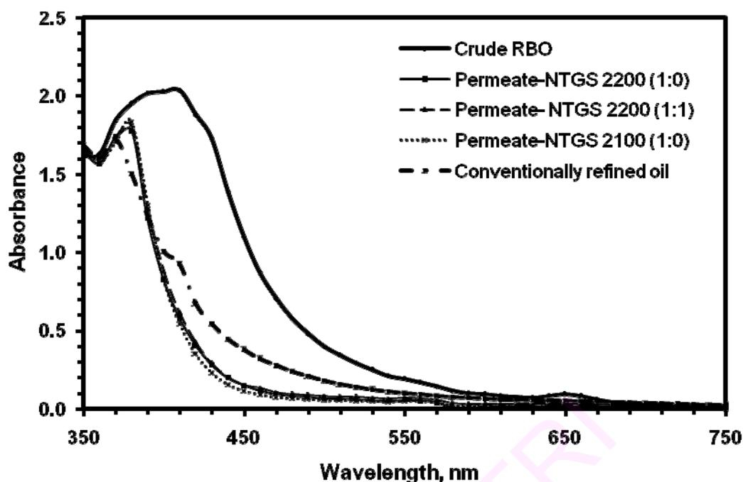
**Fig. 5.5** Visible spectra of membrane-processed CRBO (lot-1)
