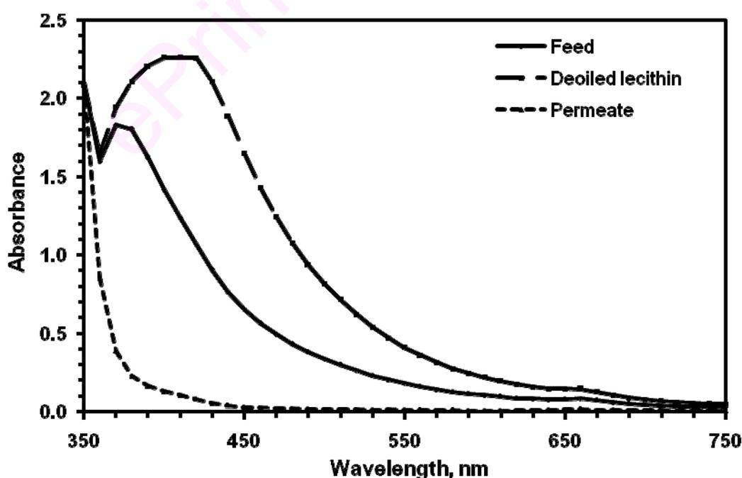
**Fig. 8.2** Visible spectra of rice bran lecithin during the membrane deoiling process (discontinuous diafiltration)
