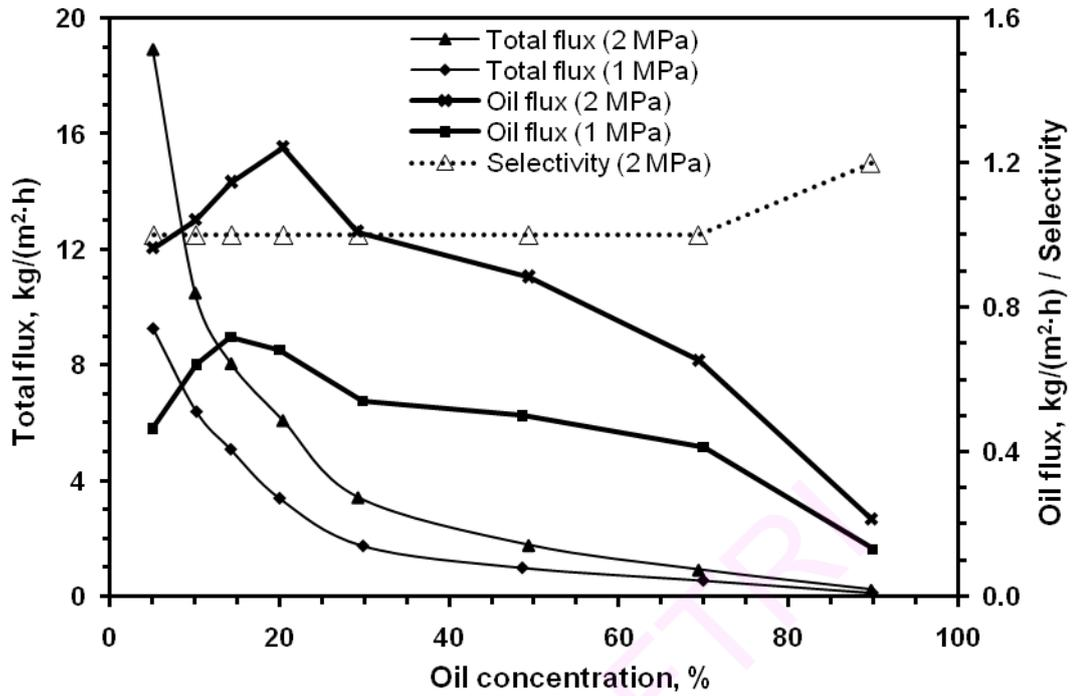
Fig. 4.4 Effect of dilution on selectivity and total and oil flux of SFO at two different pressures
