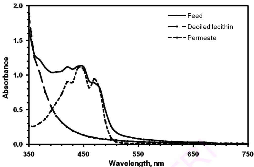
**Fig. 8.1** Colour reduction in soy lecithin during membrane deoiling process (simulated continuous diafiltration)
