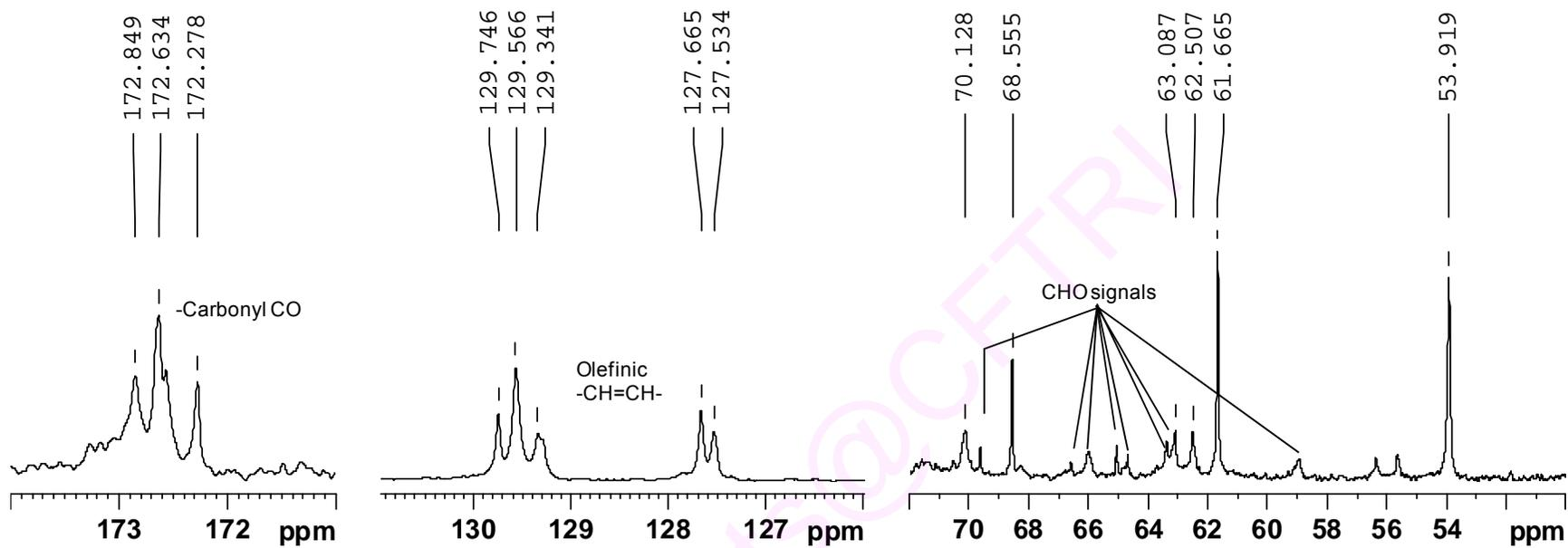
**Fig. 5.2**  $^{13}\text{C}$  NMR spectrum of the CRBO feed. ~40 mg dissolved in  $\text{CDCl}_3$ -DMSO- $\text{d}_6$  mixture was employed for recording the spectrum at 125.8 Hz. Other conditions are mentioned in the text. CHO - Carbohydrate signals.
