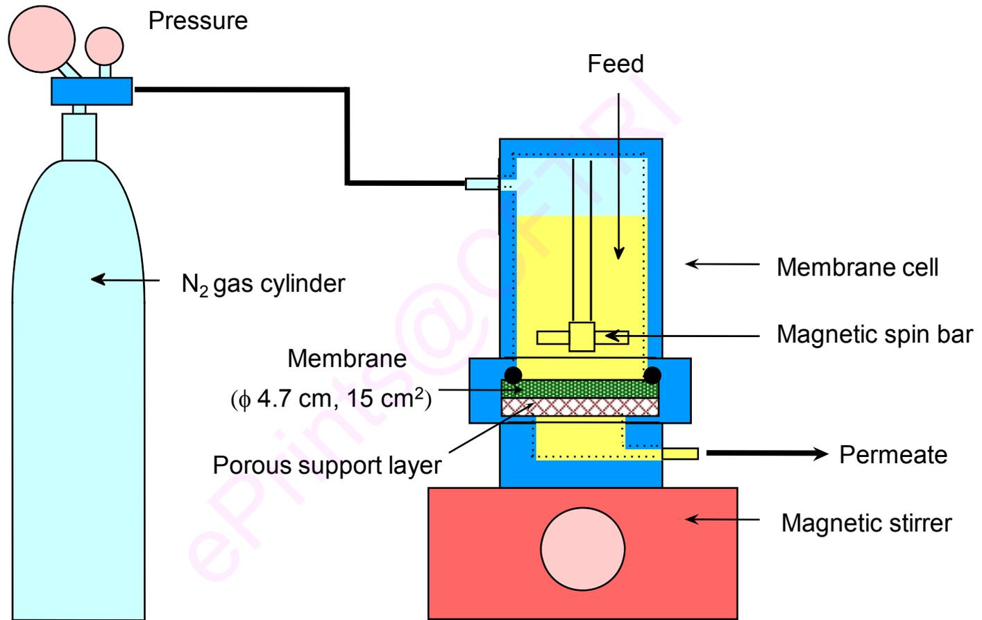
**Fig. 2.1** Self-stirred flat membrane test cell
