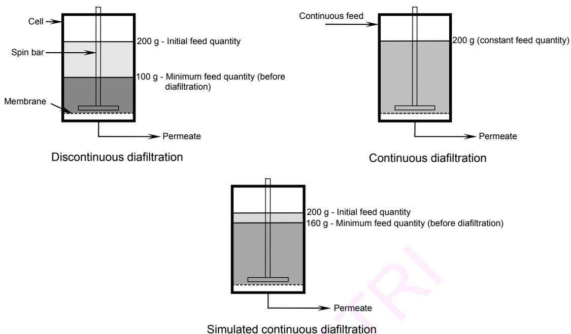
**Fig. 2.2** Diafiltration in batch membrane cell
