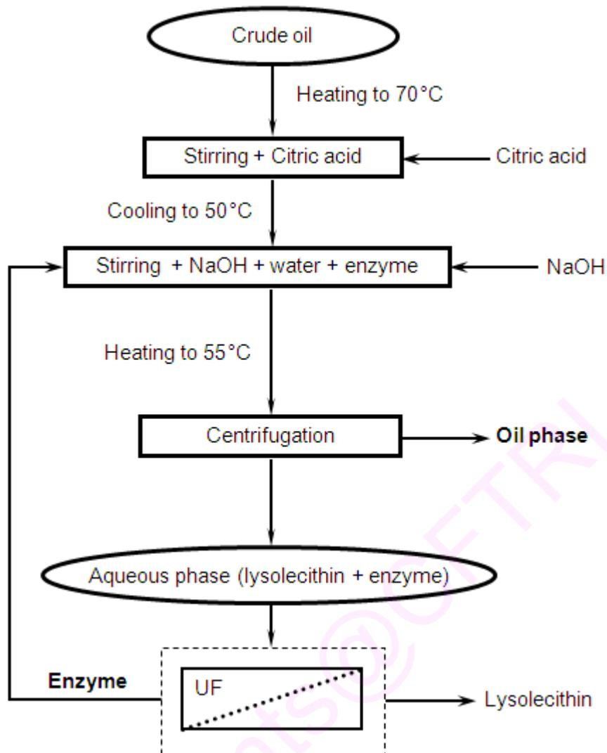
**Scheme 6.1A** Recycling of phospholipase in enzymatic degumming process
