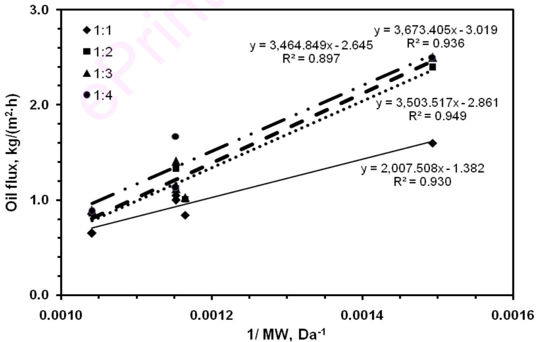
**Fig. 4.7** Relation between oil flux and average molecular weight of TG under hexane-diluted conditions
