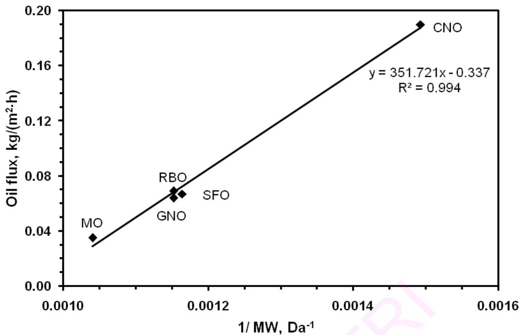
**Fig. 4.3** Relation between oil flux and average molecular weight of TG of various vegetable oils
