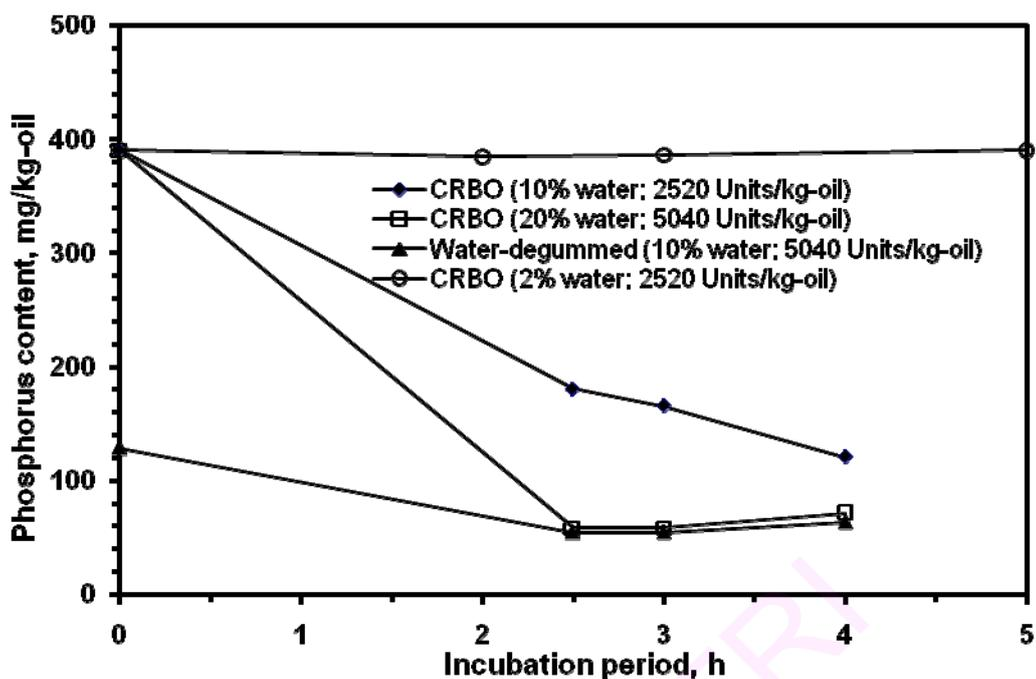
**Fig. 6.2** Reduction in phosphorus content in CRBO as a function of incubation time during enzymatic degumming in solvent phase (hexane/petroleum ether)
