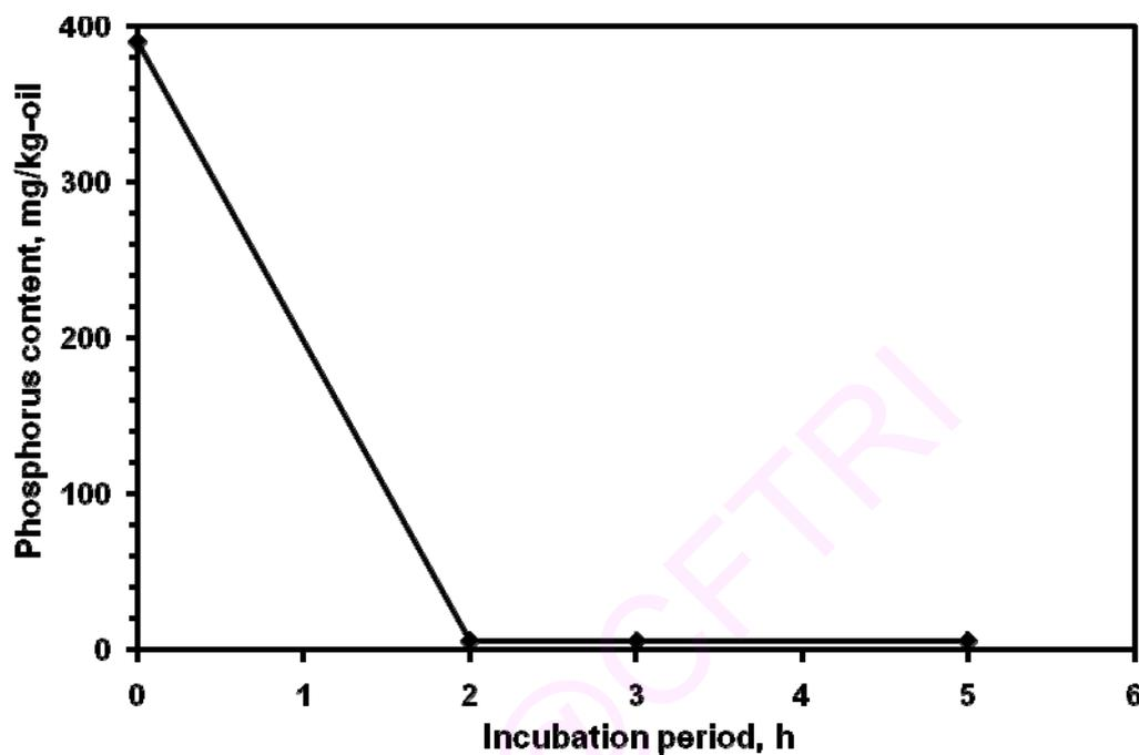
**Fig. 6.1** Reduction in phosphorus content in CRBO as a function of incubation time during enzymatic degumming (water addition 2%; enzyme dosage 2520 Units/kg-oil)
