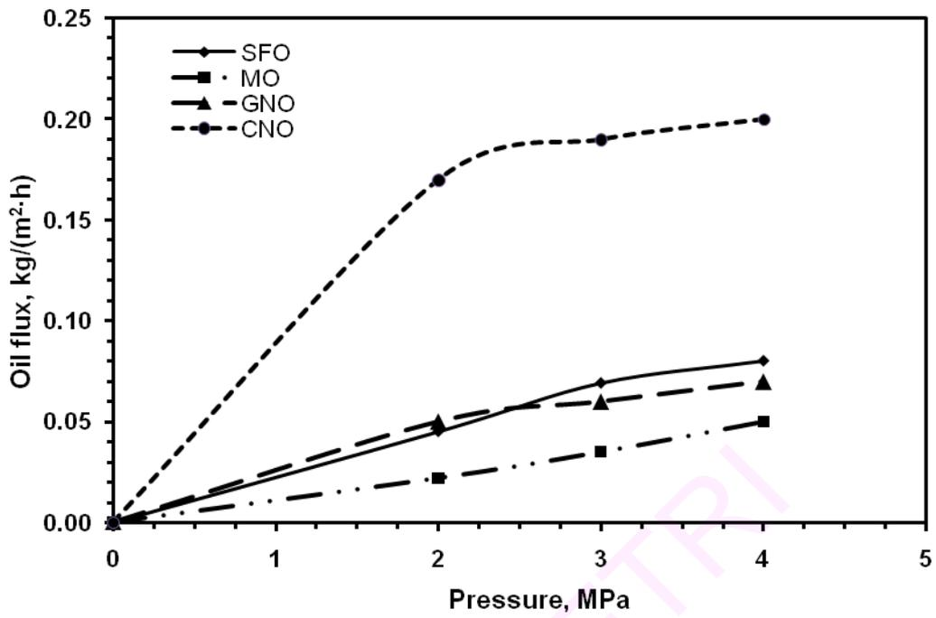
Fig. 4.1 Effect of pressure on oil flux of undiluted vegetable oils
