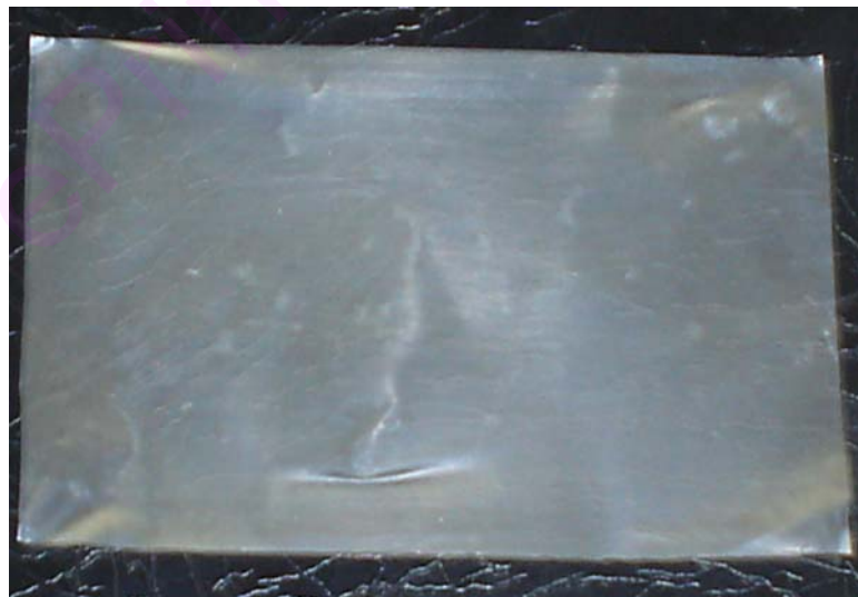
Figure 2.25: Polyhydroxyalkanoate produced by B. flexus formed into a film after chloroform casting method.
