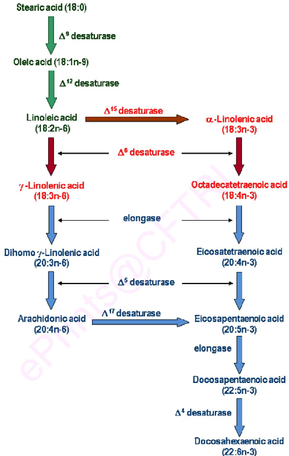
**Figure 3.** The general biochemical pathway of *in vivo* synthesis of PUFAs in various organisms. Green arrows represent reactions that are very common in higher plants; Red arrows represent reactions that occur only in a few plants; Blue arrows represent reactions that occur only in some lower organisms. (Source: Alonso and Maroto, 2000).
