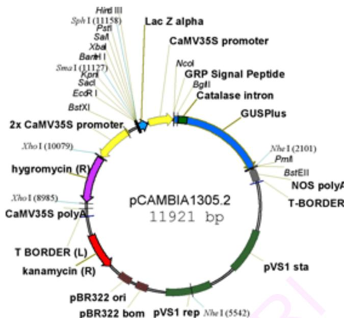
**Figure 5. Diagrammatic representation of the binary vector pCAMBIA 1305.2**
