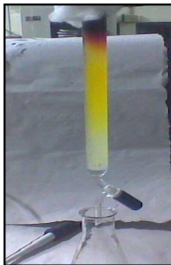
Figure 42. Silica gel column chromatography for the separation of ankaflavin (pigment).
