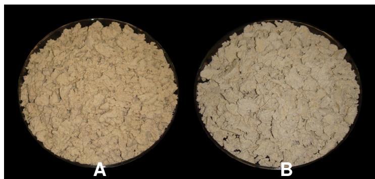
Fig 2.3 Harvested and lyophilized biomass of M. alpina used for extraction A-Wet biomass, B-Lyophilized biomass
